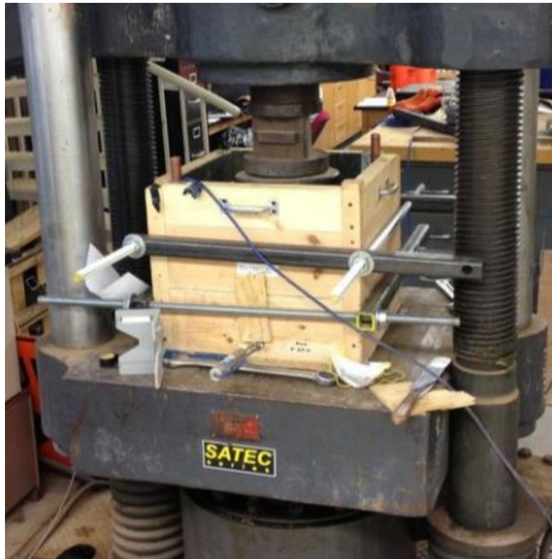
Figure 3.13: The test box filled with soil under load frame compression
