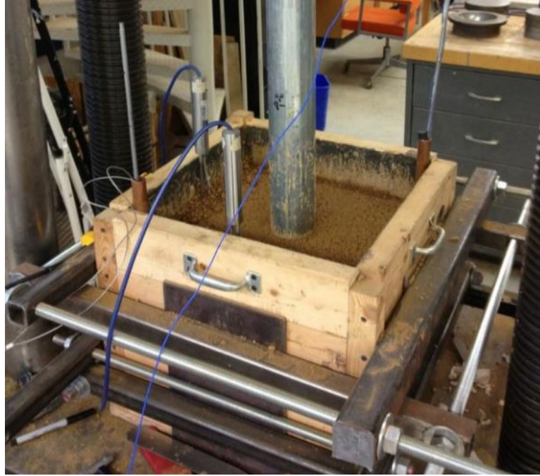
Figure 3.15: A shelly tube being driven into the compressed soil by the load frame
