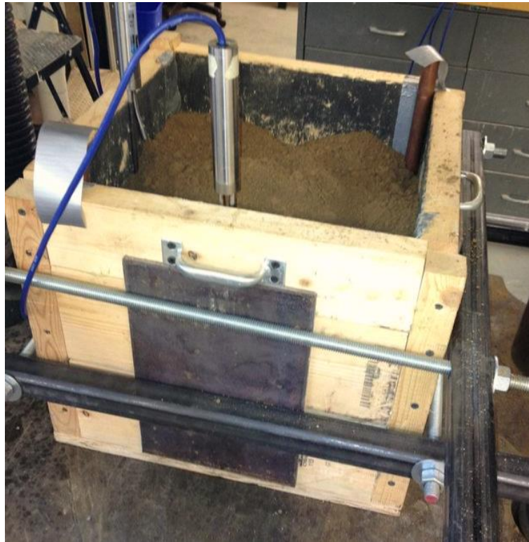
Figure 3.12: Partially loaded box with pressure plates and copper tubes in place
