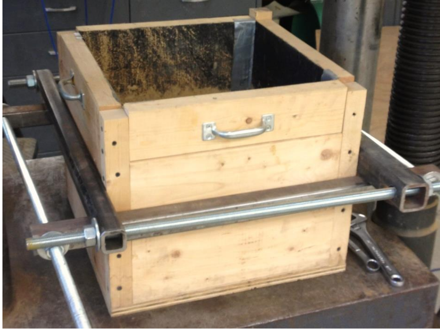
Figure 3.11: Testing box with bracing
